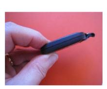
5. Next Place bottom part of the shell over the top part and press it till it closes firmly.
