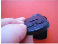
5. Press Silicone pad in till buttons are correctly positioned in respective holes of the plastic shell. Buttons should be positioned in cut outs of plastic shell as in the picture on the left.
